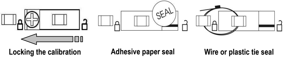
Figure 4-1. Locking and Sealing the Calibration Lock Switch.
